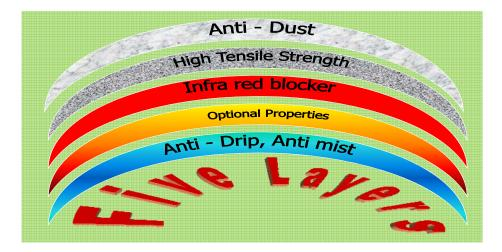
Despite the apparent simplicity of the process, years of experience are required to achieve products of high quality. The advantages of 5 layer co-extrusion over mono-extrusion (single layer extrusion) and 3 layer extrusion are:
